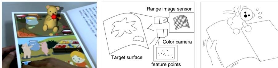
**Figure 1.** Left figure shows an AR picture book made of hard carton boards, middle figure is configuration of the proposed system, and right one is an example of the interaction system.
