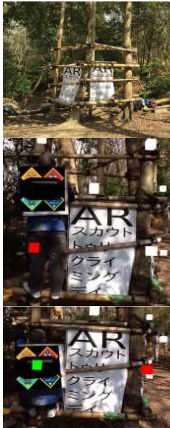
Figure 3: Tree Climbing scenario (top) and screenshots of the system (middle and bottom). The user instructs the climber the direction of the movement. Red cubes indicate where the climber goes next; green shows successfully visited points.
