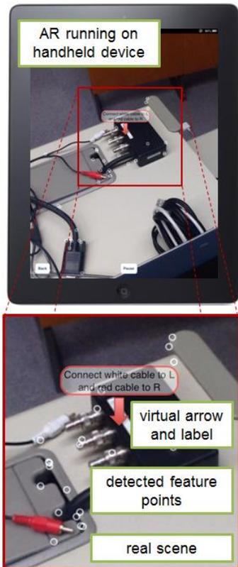
Figure 1: The HAR system we tested in [8]. The system runs on a tablet PC and enables the users to add virtual labels onto the real scene. More information about this HAR system, and our other HAR interactions can be found in [9].
