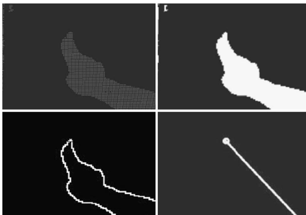
**Fig. 7** Detect finger-pointing position from outlier image. *Upper-left* an outlier image, *upper-right* a result of labeling operation, *lower-left* outline of a hand area, *lower-right* estimation to fingertip direction
