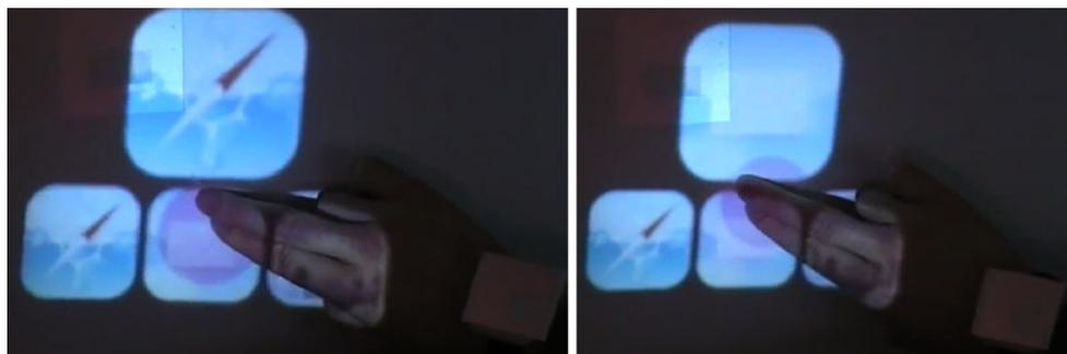
**Fig. 5** Interaction by tapping on the wall. The biggest icon changes according to the tapping position
