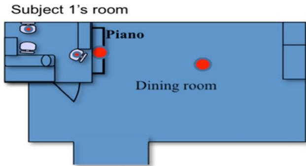
**Fig. 8** Data acquisition via sensors. *Red dots* mark the placement of the four location sensors
