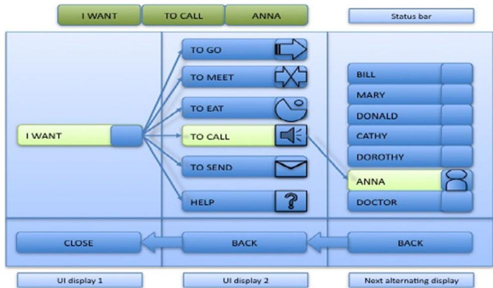
**Fig. 3** Prototype system, which provides tapping interface on a wearable computer
