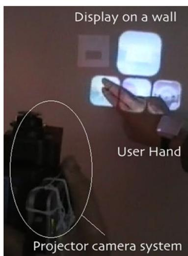
**Fig. 6** Projector camera system detects markers on the wall and user's wrist and input signal by acceleration sensor
