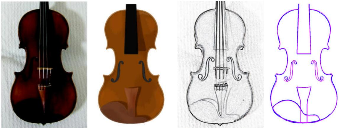
(a) Violin (photo) (b) With log-aesthetic curve (c) Outline (d) B-spline (blue) and log-A curve (red)
