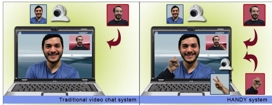
Figure 1 Traditional video chat system (left) and HANDY system (right) components.
